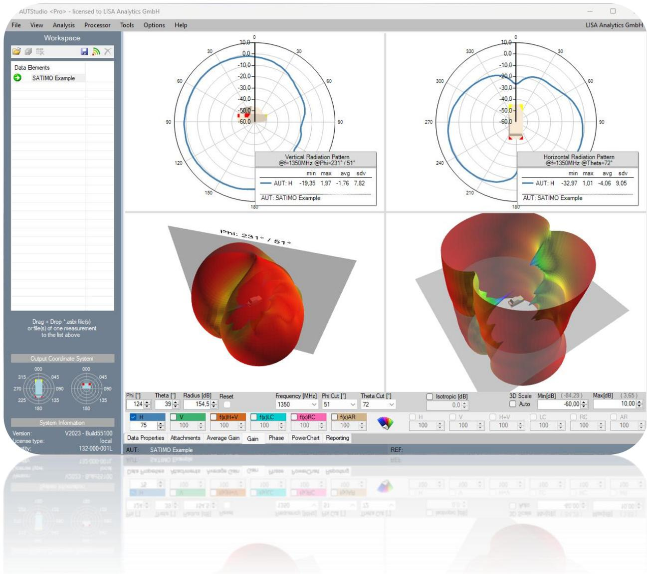
An interactive “on the fly” 3D view algorithm brings the visualization part of a measurement system or simulation tool to the engineer’s desktop.
